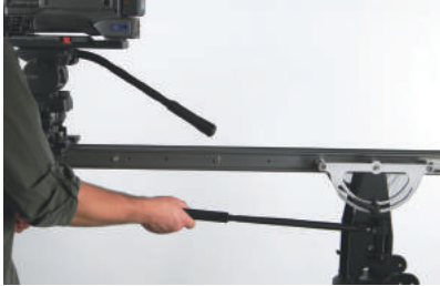
FIG 49. You may need to adjust the length of the parallel arm to adjust framing.
