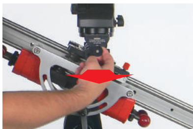
FIG 32. You will have to pull the black circular adjustment knob with great force to achieve this.
