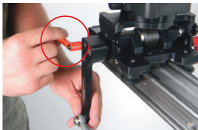
FIG 48. The lever with red 'kip' handle should be perpendicular to the rail. This will ensure parallel camera movement to the ground.
