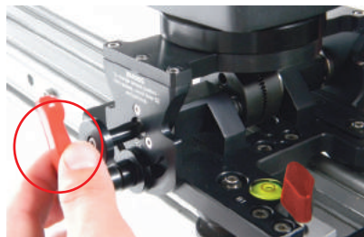
FIG 52. Release the red 'kip' handle underneath the black adjustment knob.
