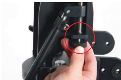
FIG 46. Turn the knob on the focal point adjustment to reposition the end of the parallelogram arm so that it is on the top of the adjustment.
